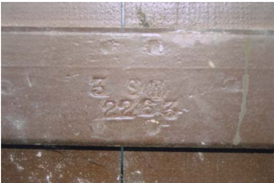
The boat number assigned to MTB 486/Sungo by the British Powerboat Company, "2263". The other symbols "3 SW" above are the individual panel position identifiers.
