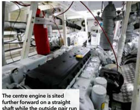
The centre engine is sited further forward on a straight shaft while the outside pair run
