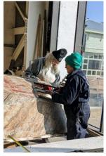
**CMB4 Replica build** – There seems to be more bits and bobs than you can shake a stick at these days. Below left Steve B is nearing the end of this particular torpedo launch control ring before getting it painted in black 'Cast' paint.
