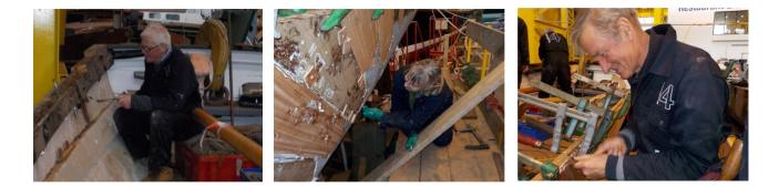
Above left a close -up of Jeremy wielding his spanner as he removes some crabby inwale sections. Above middle Roz R is pulling in the bottom end of one of our new planks and finally Hamo cleaning up surplus glue from the new planking on the port side. It is probably appropriate that this article started and ended with Hamo T working his magic as he extends the Thorneycroft boat building history.
