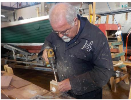
Above left Mike S is trialling a jointing process for the rowlock chock/ wash-board, here he is trialling twin dowels having already knocked the biscuit joints on the head. Shortly after this we decided to revert to 'Simple' and do away with all fiddly bits and go for a bog -standard butt joint. KISS!
