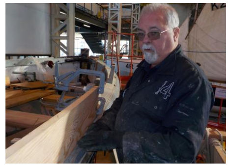
Above left Mike S is trialling a jointing process for the rowlock chock/ wash-board, here he is trialling twin dowels having already knocked the biscuit joints on the head. Shortly after this we decided to revert to 'Simple' and do away with all fiddly bits and go for a bog -standard butt joint. KISS!
