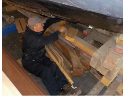
Above left Ian P is making himself comfortable in the bilges as he, Hamo T and Steve B are removing some of the old engine bearers to make way for the rest of the floors to take the bottom boards. Above Middle Hamo is stretching out under the boat as he receives some of the engine bearer bolts being driven through by Ian. Finally Hamo is over far right dry fitting two of the new floors.
