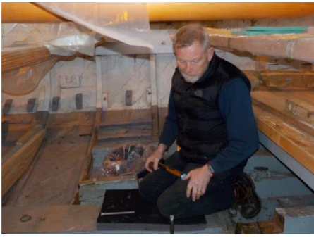
Above left Ian P is making himself comfortable in the bilges as he, Hamo T and Steve B are removing some of the old engine bearers to make way for the rest of the floors to take the bottom boards. Above Middle Hamo is stretching out under the boat as he receives some of the engine bearer bolts being driven through by Ian. Finally Hamo is over far right dry fitting two of the new floors.
