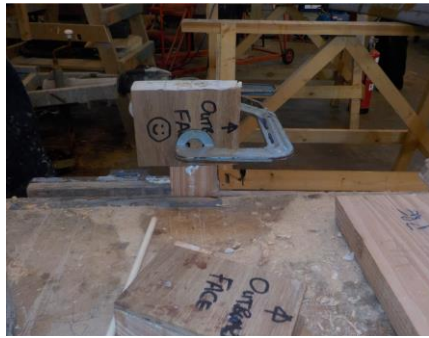
Above left Mike S is trialling a jointing process for the rowlock chock/ wash-board, here he is trialling twin dowels having already knocked the biscuit joints on the head. Shortly after this we decided to revert to 'Simple' and do away with all fiddly bits and go for a bog -standard butt joint. KISS!
