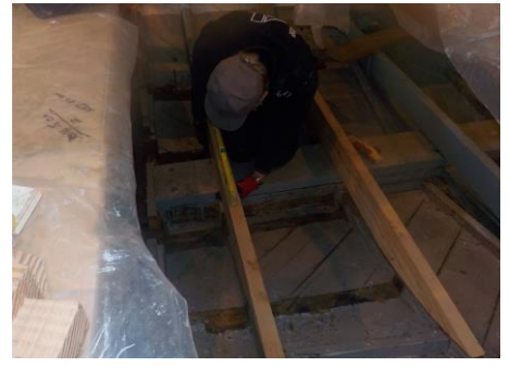
Above left Ian P is making himself comfortable in the bilges as he, Hamo T and Steve B are removing some of the old engine bearers to make way for the rest of the floors to take the bottom boards. Above Middle Hamo is stretching out under the boat as he receives some of the engine bearer bolts being driven through by Ian. Finally Hamo is over far right dry fitting two of the new floors.
