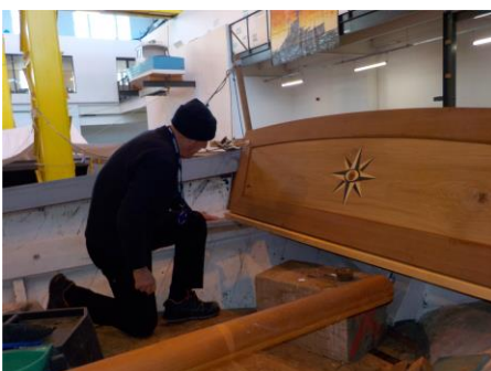
Above left Mike S is trialling a jointing process for the rowlock chock/ wash-board, here he is trialling twin dowels having already knocked the biscuit joints on the head. Shortly after this we decided to revert to 'Simple' and do away with all fiddly bits and go for a bog -standard butt joint. KISS!
