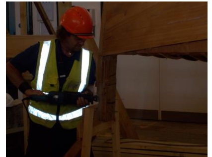
are fitting the main lifting straps. Having taken the weight on the crane Tiger is underneath with his sabre saw cutting away at the building blocks and finally above right he cuts through the stem leaving the boat to 'float away' up to the ceiling.
