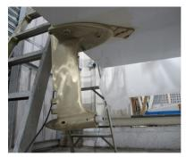
Below left is a photo of the bronze cast rudder, with the stern fitting shown in the middle photo below far right are some of
