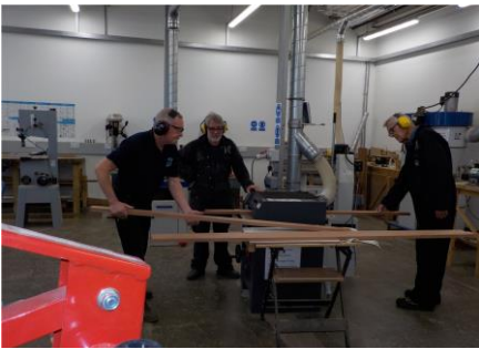
Above left Ian P, Mike F and Steve B are machining some stock timber to make the torpedo trough bottom board support frame whilst above middle With Ian B they are making a pattern of the cockpit to make a bending jig to laminate the parts of the coaming. Above right Steve B and Fred A are gluing and screwing the 'ladder' section of trough bottom board support frame. Below left Ian P and Mike F are machining some 4mm laminates for the cockpit coaming along with Ian B middle below. Below far right is an overall shot of the boat with the torpedo trough bottom board support ladder as a trial fit.
