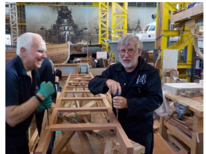
Above left Ian P, Mike F and Steve B are machining some stock timber to make the torpedo trough bottom board support frame whilst above middle With Ian B they are making a pattern of the cockpit to make a bending jig to laminate the parts of the coaming. Above right Steve B and Fred A are gluing and screwing the 'ladder' section of trough bottom board support frame. Below left Ian P and Mike F are machining some 4mm laminates for the cockpit coaming along with Ian B middle below. Below far right is an overall shot of the boat with the torpedo trough bottom board support ladder as a trial fit.
