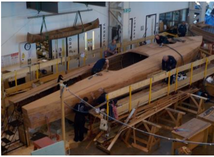
Above left a shot overall showing the boat with all her planking, above middle Ian P is down and dirty drilling out the pilot holes for the final copper nailing, I think from his body language he is thinking "thank goodness, nearly there, only a few more mouthfuls of sawdust and we can call it a day". Above right Roz is skulking under the after decking clearing out all the surplus glue drips and filling any random holes.
