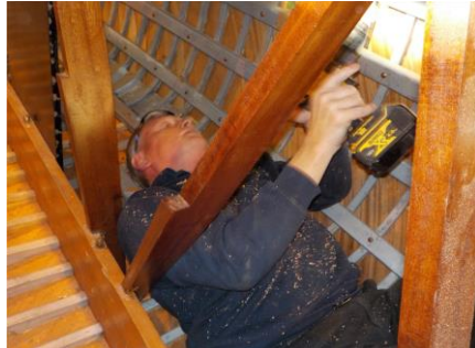
Above left a shot overall showing the boat with all her planking, above middle Ian P is down and dirty drilling out the pilot holes for the final copper nailing, I think from his body language he is thinking "thank goodness, nearly there, only a few more mouthfuls of sawdust and we can call it a day". Above right Roz is skulking under the after decking clearing out all the surplus glue drips and filling any random holes.
