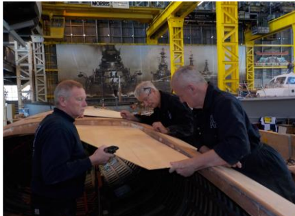
Above left Ian P, Mike F and Steve B are machining some stock timber to make the torpedo trough bottom board support frame whilst above middle With Ian B they are making a pattern of the cockpit to make a bending jig to laminate the parts of the coaming. Above right Steve B and Fred A are gluing and screwing the 'ladder' section of trough bottom board support frame. Below left Ian P and Mike F are machining some 4mm laminates for the cockpit coaming along with Ian B middle below. Below far right is an overall shot of the boat with the torpedo trough bottom board support ladder as a trial fit.
