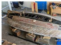
doing her real job), are on the last knockings of removing the hog, keel and secondary keel from the boat. Whatever you do make sure nobody sneezes around the dory, otherwise Steve wont have a boat to rebuild. Above middle, Pauline has just wedged open the joint and above right the whole assembly has been taken out.
