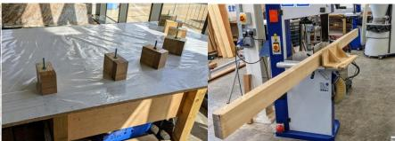
Above middle photo shows the lofting board re-configured as a moulding board covered in polythene sheet to stop any glue sticking to it when Steve starts gluing up the laminates. Firstly, he needs to machine up some laminates from solid oak stock, above right they have just set up the bandsaw to split down an oak plank into 5mm thick laminates.
