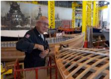
that the foredeck timbers are fair and true whilst lan P and Steve B prepare the king plank which will run from the stem back along the centre of the foredeck to the forward hatch and on back to the cockpit edge. Below left lan and Steve B are fitting the king plank in place with resin and polymer nails with Tim D making sure that the plank is true as it comes up to
