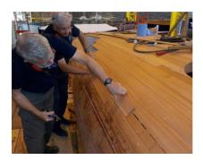
Below left Steve B and Mike F are just putting in the last nail in the last plank on the port side, next photo in the middle shows the whole of the boat with virtually all her first layer planking complete, just a couple of small spaces forward on the foredeck. And finally, below right the second layer planking is also nearing completion as the guys work on the complex multi curves of the foredeck fighting the 9mm planking with a mind of its own.
