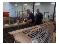
torpedo trough edges from which we will work out and along. The next two photos show these first planks in place.—Below left John and Mike F are gluing up number two plank along the port side quarter. Next below middle Tim D is making sure
