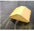
Launch's Emergency Float Rope locker. Below we can see it being given the 'Float Test', as you can see it is upright and stable as it faces the full onslaught of Portsmouth Harbour in a Spring Tide. The photo was taken just
