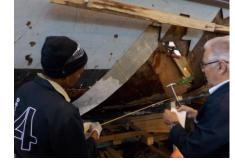
photo over right John C and Fay are tacking the calico in place
