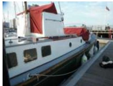
Over left after a couple of day's work the cracks have gone but so has the varnish and at this stage she has had her after coach roof rubbed down, filled and undercoated along with an undercoated Starboard side deck and a freshly painted cabin
