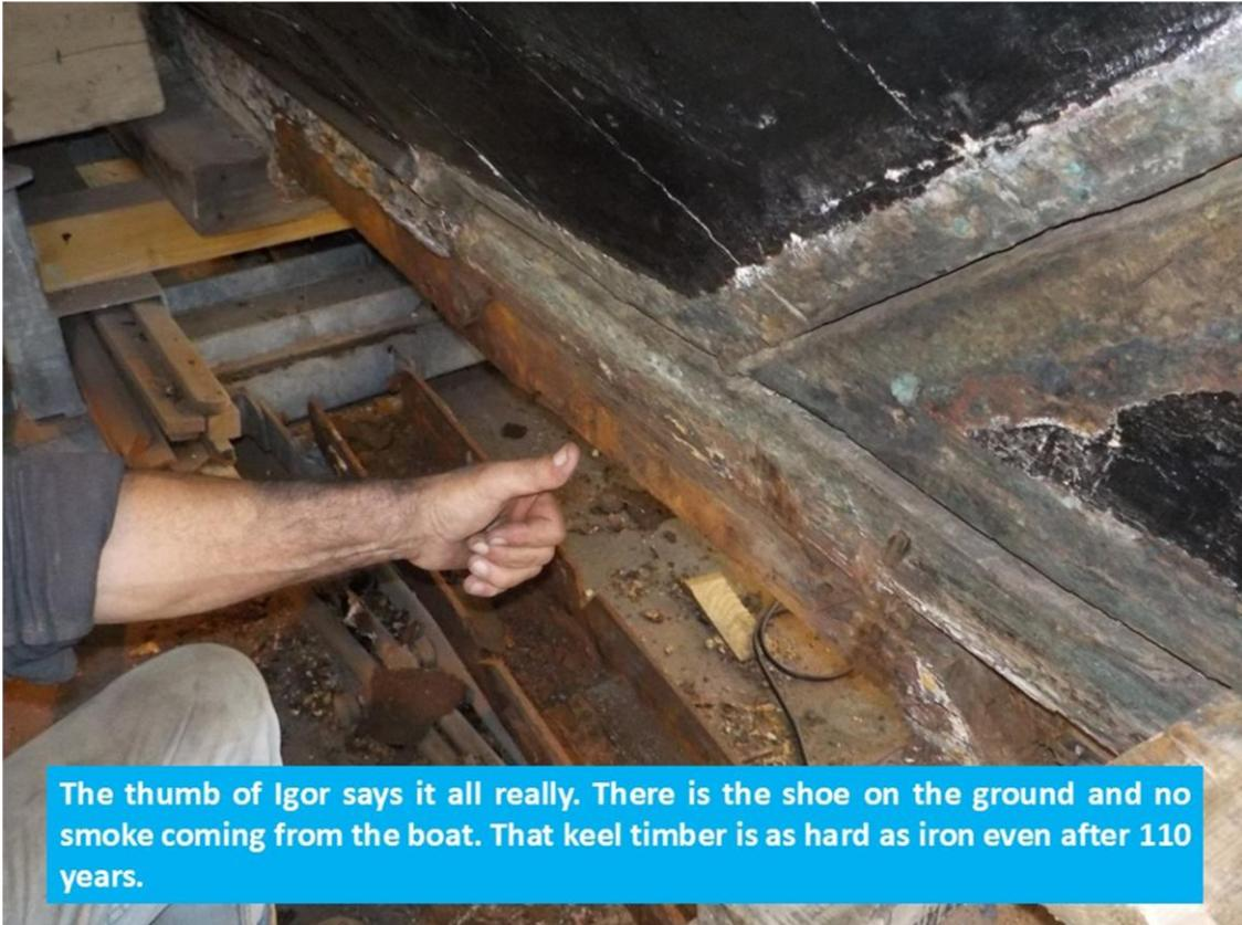
The thumb of Igor says it all really. There is the shoe on the ground and no smoke coming from the boat. That keel timber is as hard as iron even after 110 years.
