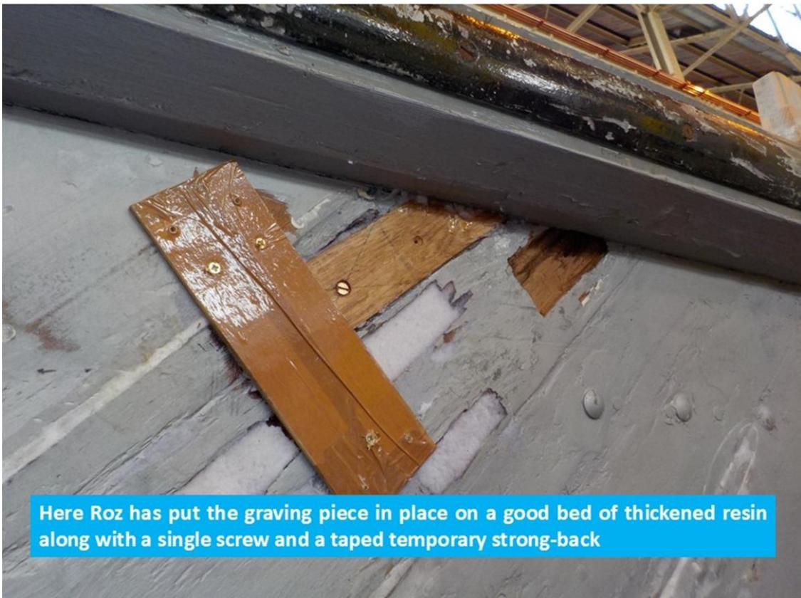
Here Roz has put the graving piece in place on a good bed of thickened resin along with a single screw and a taped temporary strong-back
