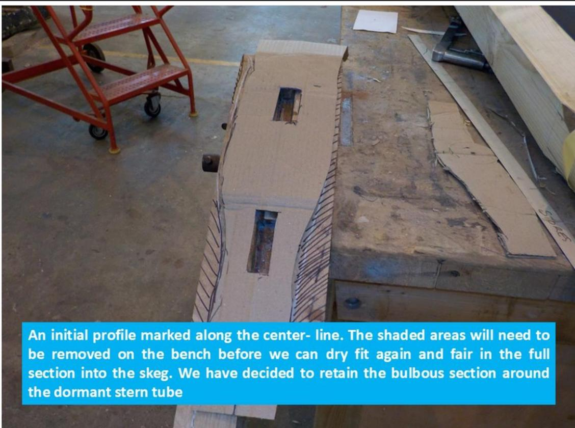
An initial profile marked along the center-line. The shaded areas will need to be removed on the bench before we can dry fit again and fair in the full section into the skag. We have decided to retain the bulbous section around the dormant stern tube
