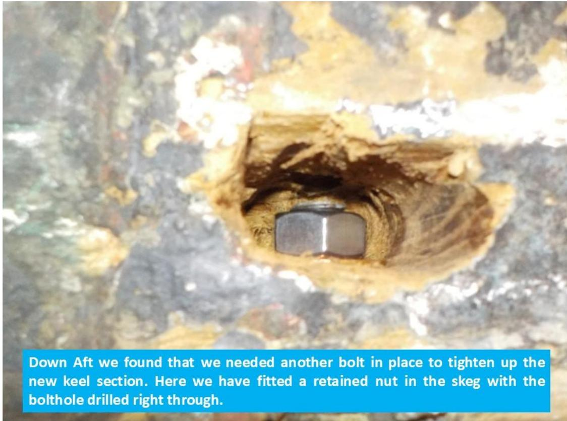
Down Aft we found that we needed another bolt in place to tighten up the new keel section. Here we have fitted a retained nut in the skeg with the bolthole drilled right through.
