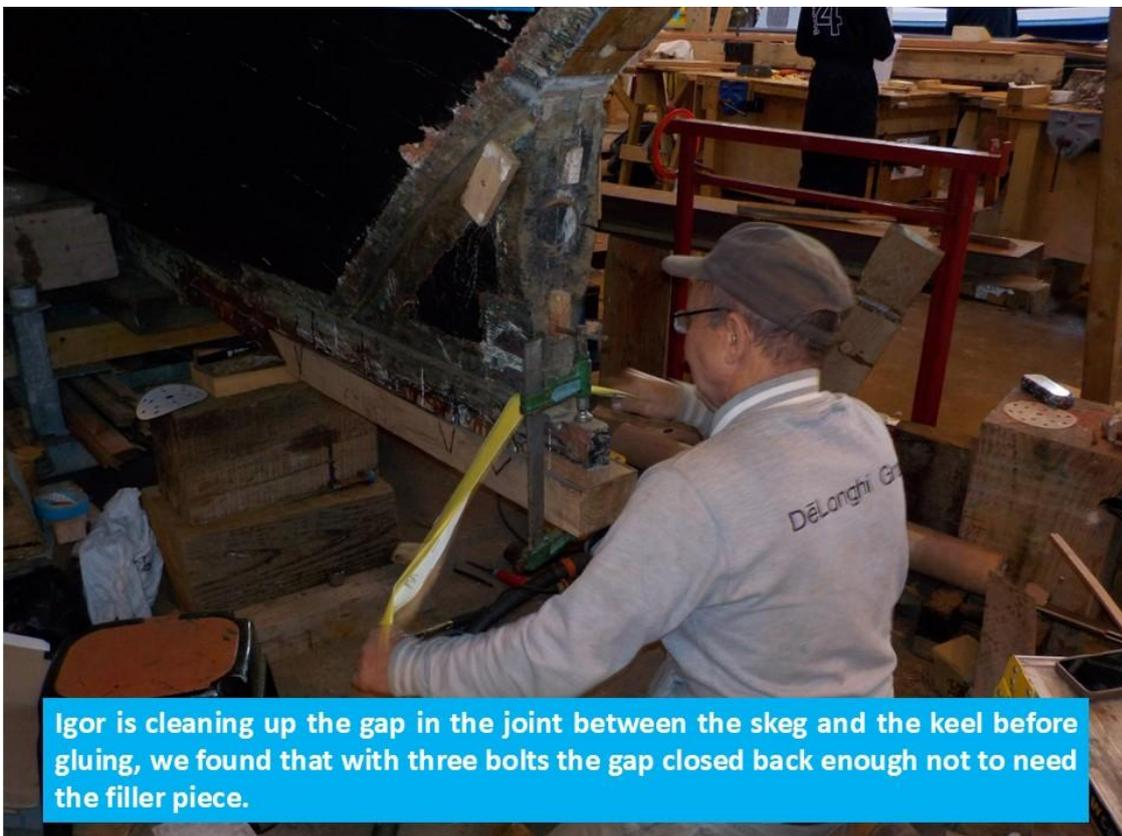
Igor is cleaning up the gap in the joint between the keel and the skag before gluing, we found that with three bolts the gap closed back enough not to need the filler piece.
