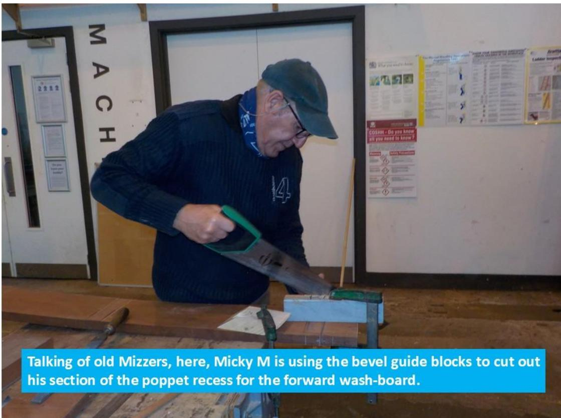
Talking of old Mizzers, here, Micky M is using the bevel guide blocks to cut out his section of the poppet recess for the forward wash-board.
