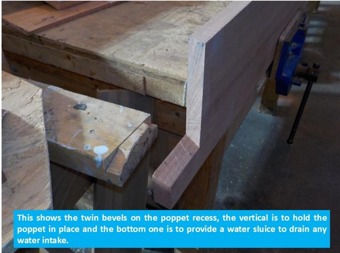
This shows the twin bevels on the poppet recess, the vertical is to hold the poppet in place and the bottom one is to provide a water sluice to drain any water intake.
