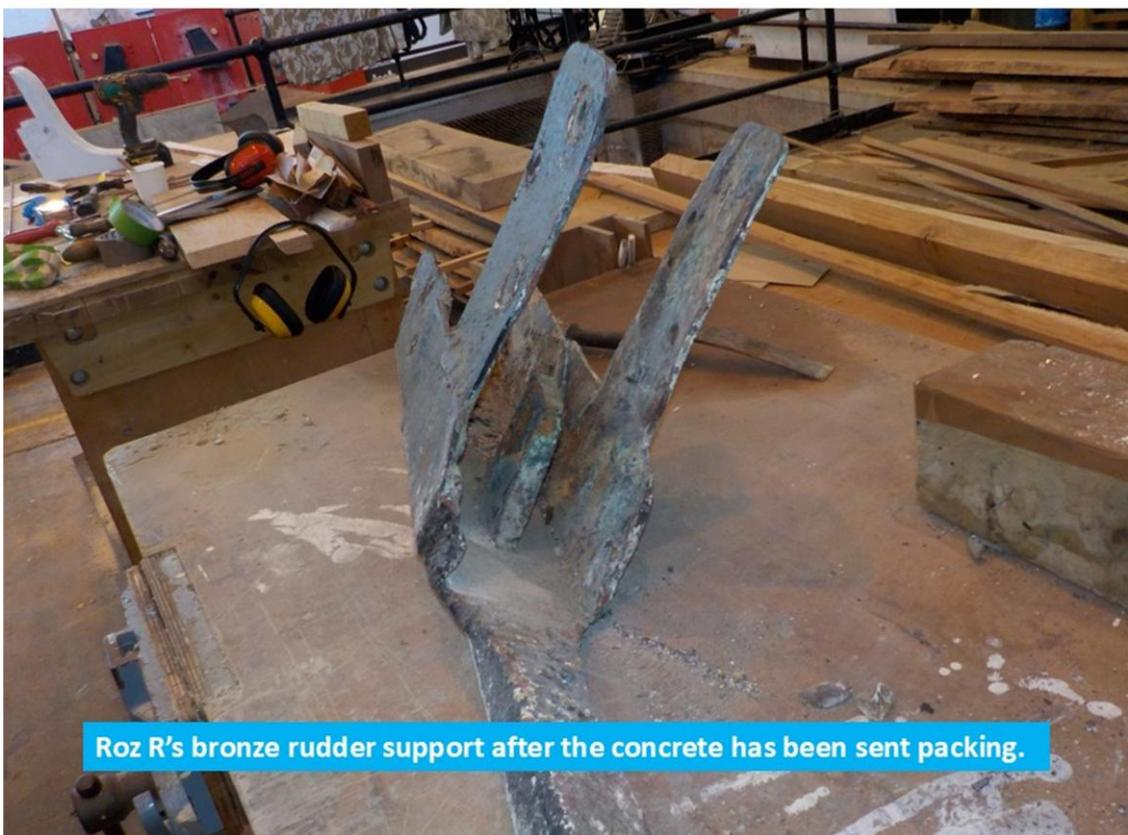
Roz R's bronze rudder support after the concrete has been sent packing.
