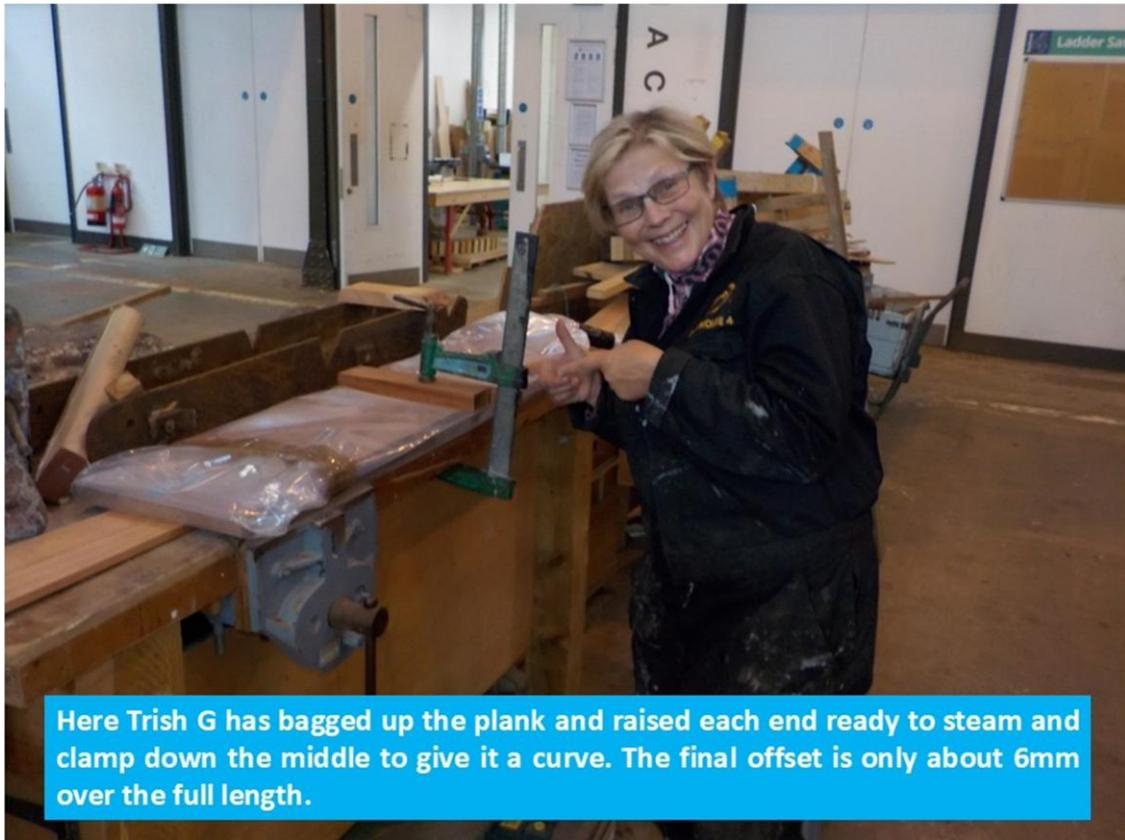
Here Trish G has bagged up the plank and raised each end ready to steam and clamp down the middle to give it a curve. The final offset is only about 6mm over the full length.
