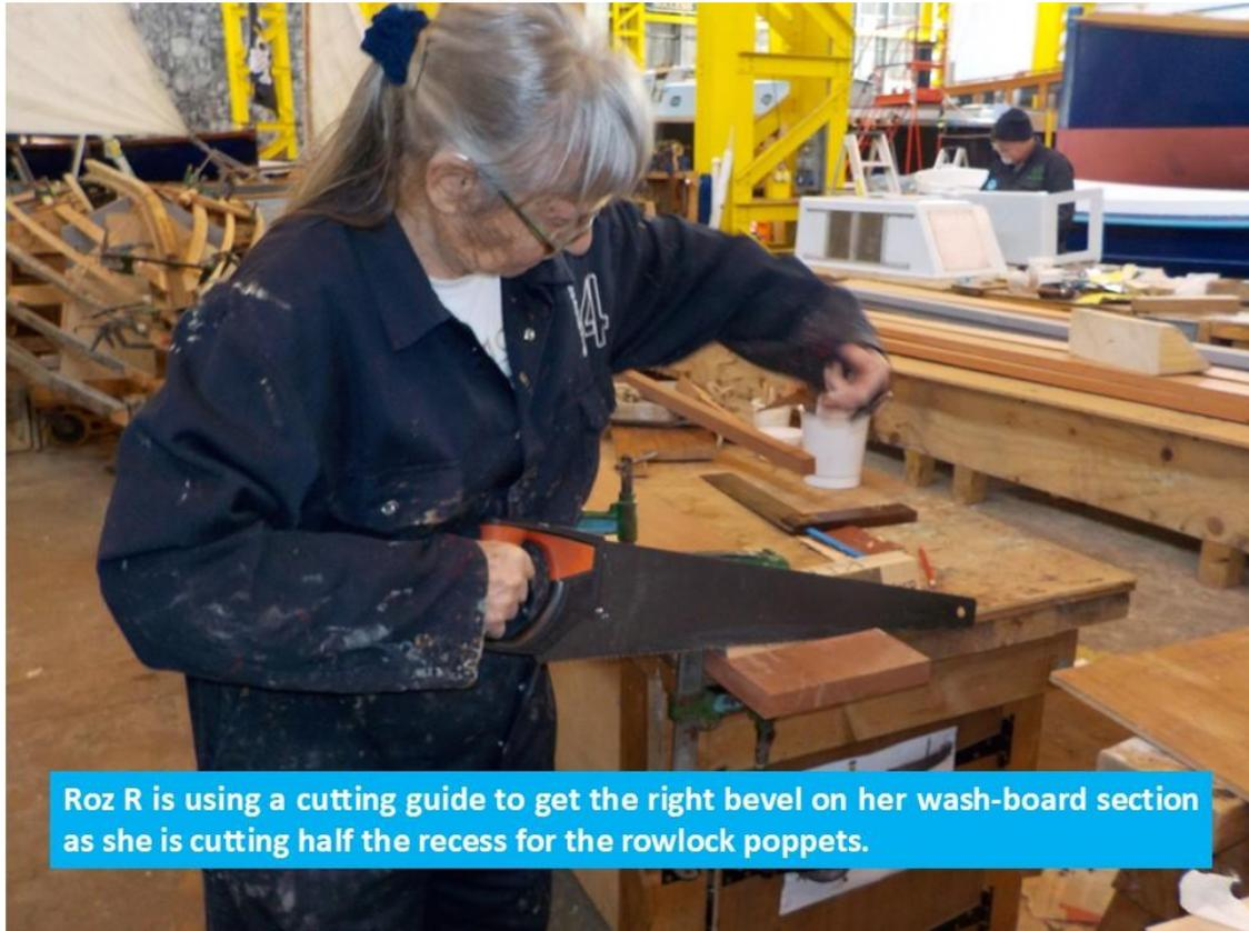
Roz R is using a cutting guide to get the right bevel on her wash-board section as she is cutting half the recess for the rowlock poppets.
