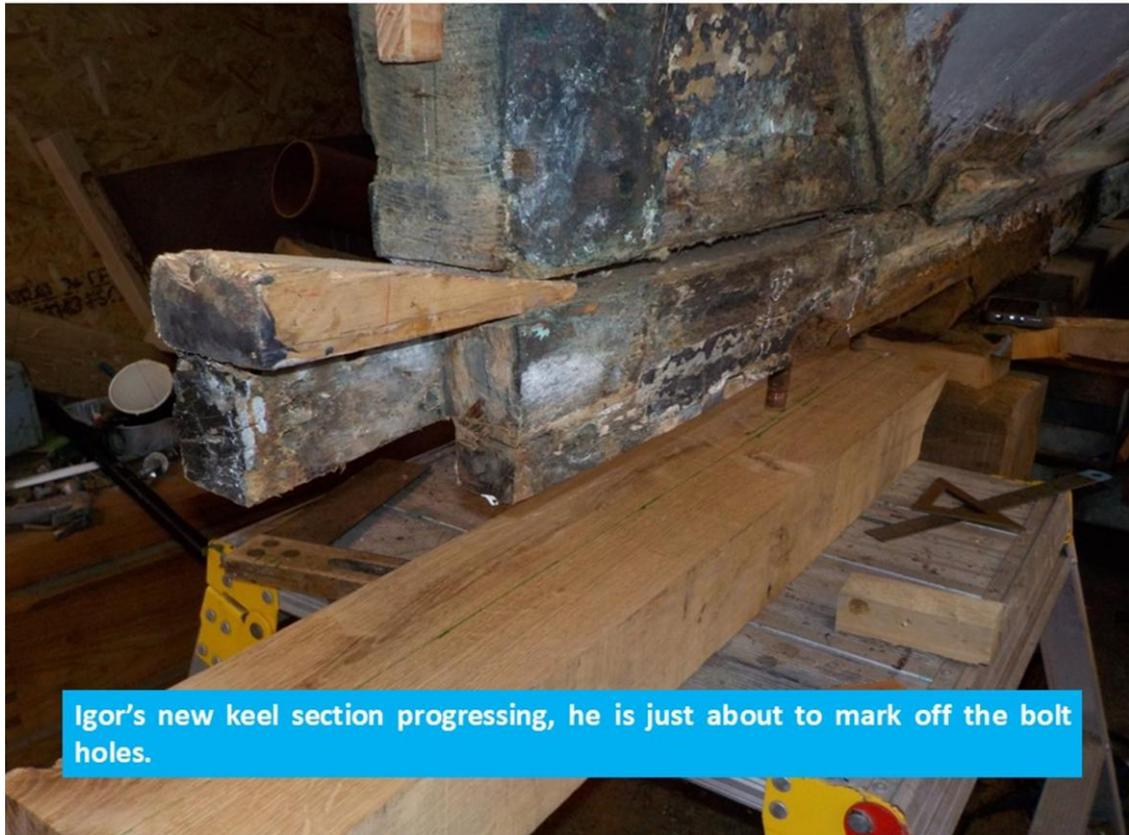
Igor's new keel section progressing, he is just about to mark off the bolt holes.
