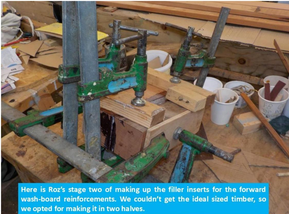
Here is Roz's stage two of making up the filler inserts for the forward wash-board reinforcements. We couldn't get the ideal sized timber, so we opted for making it in two halves.
