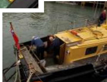
of the photo with Knotty Tony and Fisherman Pete down aft working on the steering lines. The rudder had become quite tight over the months and the choice was to send Danny on a 'Mr Universe' course or get it sorted out. In the photos below the side steering sheave blocks are being removed so that the sheaves can be serviced. Alan B (2)
