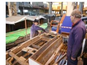
assembly job is to complete the after deck and tiller flat which had been stripped back to basic cross beams. Dave, Whaler John and Fred
